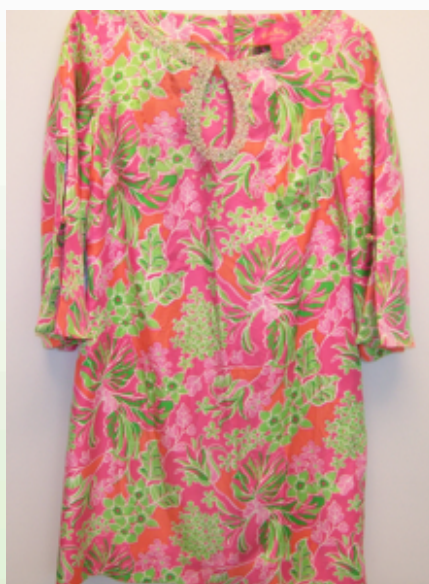
This dress had plastic trim at the neckband area that dissolved during acceptable drycleaning procedures.
