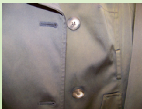
After drycleaning, there has been so much loss of black color that the coat looks goldish brown in many areas.
