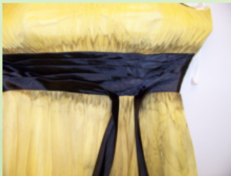
After drycleaning as labeled, the black fabric dye transfer is readily seen in this close up picture.
